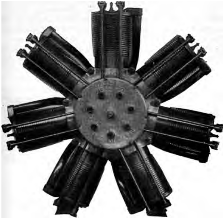
Fig. 10. Metz Seven-Cylinder Revolving Motor with Nickel-Steel Cylinders
